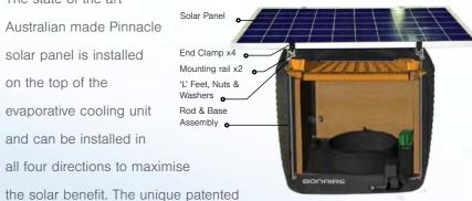
rod and clamp mounting system securely attaches the solar panel to the cooler. This design has been proven in wind tunnel testing conducted by the University of Adelaide School of Civil, Environmental and Mining Engineering. The solar panel is connected to an intelligent micro inverter that converts DC into AC power that is in turn connected to the cooler control box.
